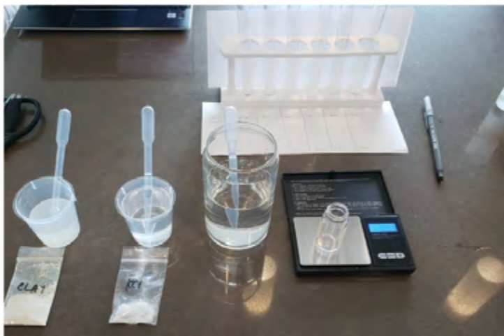
In one surfaces and colloids lab, students use a series of salt solutions to investigate the minimum concentration required to destabilize a dispersed clay particle, mimicking wastewater treatment.
