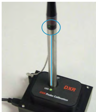
Figure 2. Probe positioned for alignment and calibration
