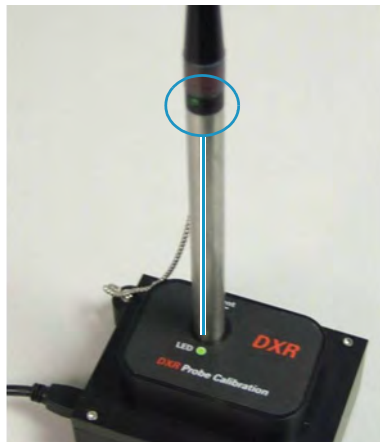
Figure 5. Probe positioned for alignment and calibration
