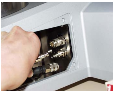
Fig. 7 - 3 Connecting the fluid circulator hoses from the accessory
