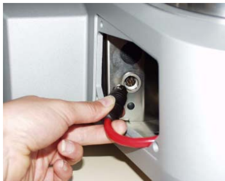
Fig. 7 - 4 Connecting the accessory cable to the instrument
