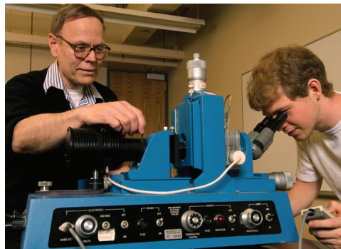
Prof. Berg works with undergraduate Keegan Wincewicz on the particle micro-electrophoresis apparatus, in this 2004 photo.
