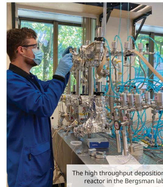
The high throughput deposition reactor in the Bergsman lab
